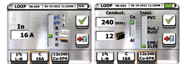
Setting of MCB/fuse type and rated current
