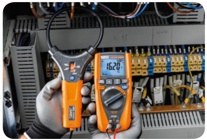
AC current measurement with flexible transducer F3000U.
