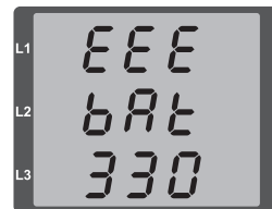
Fig. Clock / battery error number 330 (clock does not run and has to be set).
