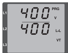
Fig. Programming mode Voltage transformer The primary and secondary currents can be changed using buttons 1 and 2 (cf. page 53).
