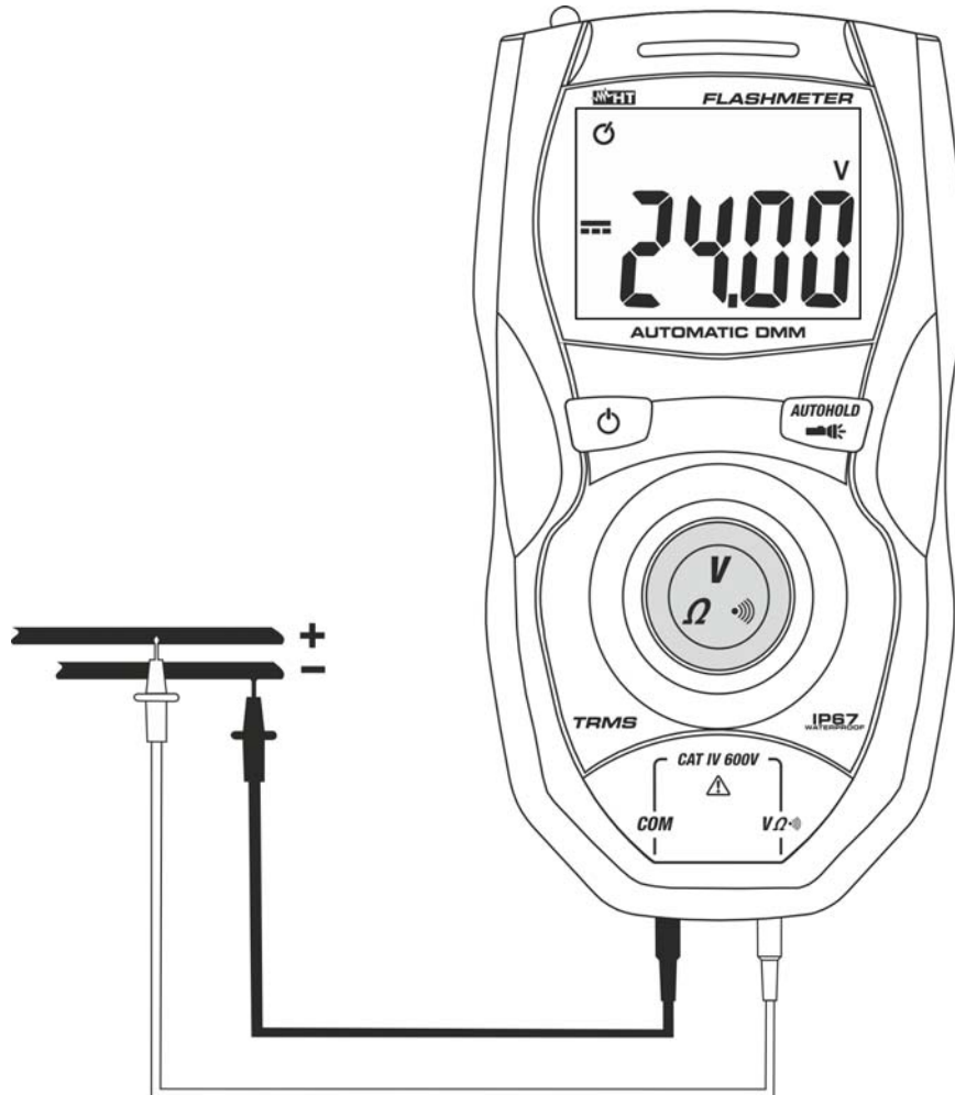
Fig. 3: Use of the instrument for DC voltage measurement
