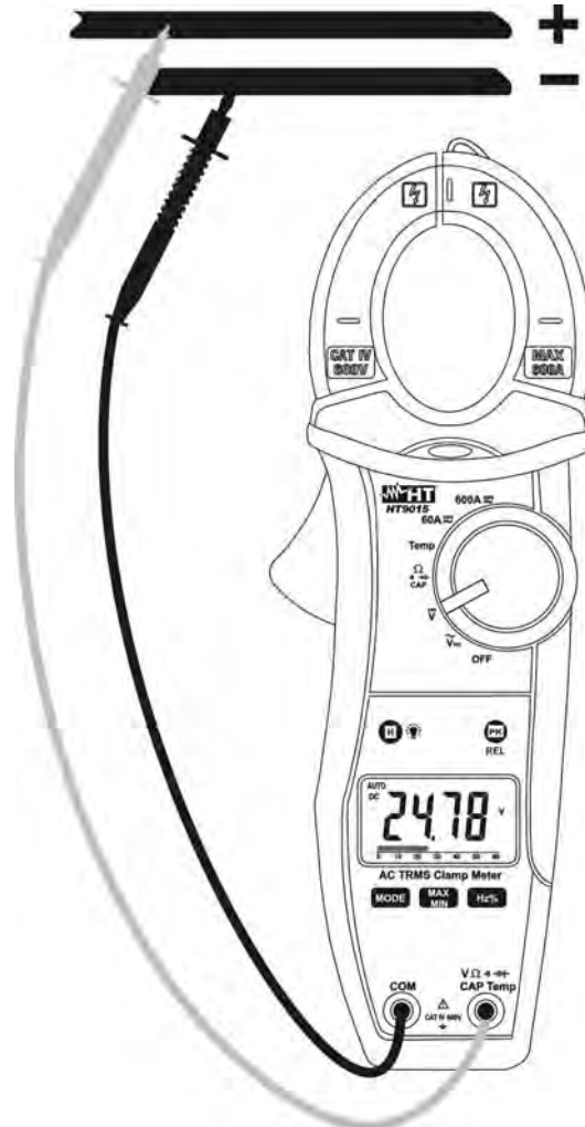
Fig. 4: Taking DC voltage measurements
