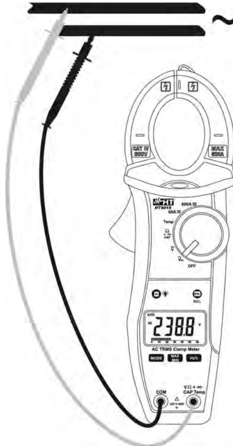
Fig. 3: Taking AC voltage measurements
