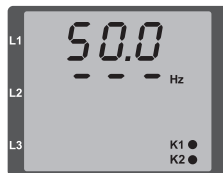
Fig. No rotation field direction detectable.
