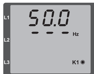
Example 2: Fig. No phase sequence determined.
