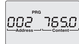
Display example 1: The primary voltage of each voltage transformer on the 4 voltage measurement inputs is 765 V.
