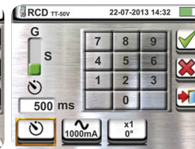
Setting of RCD delayed time
