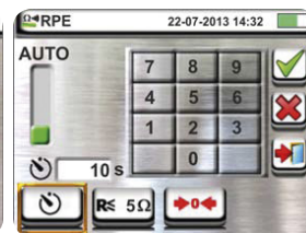
Selection of AUTO or TIMER measuring mode
