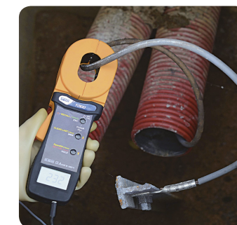
Measurement with clamp T2100
