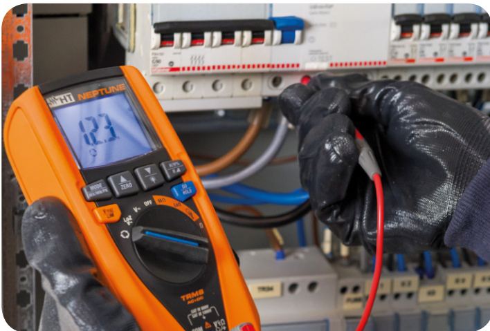
Measurement of phase sequence with one lead .
