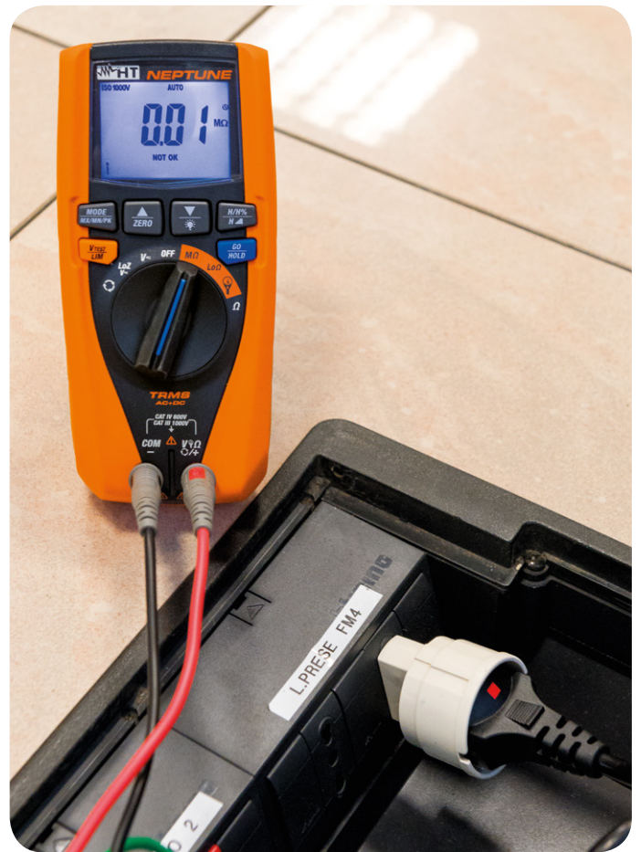
Measurement of Insulation Resistance (optional Schuko C2065 adapter).
