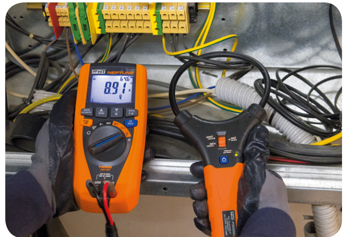
Measurement of current through flexible transducer F3000U .
