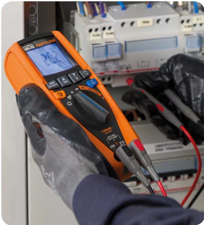
Voltage measurement with test leads.
