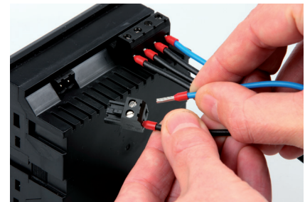
Fig.: Pluggable screw terminals for easy connection
