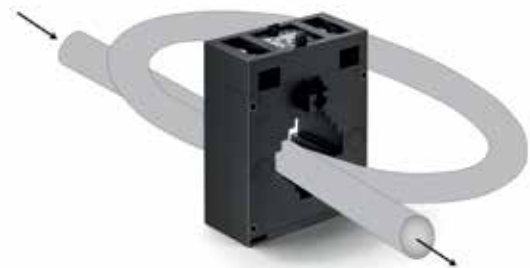
Equivalent to a transformer 100 / 5 A, I_{max} = 50 A
