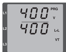
Fig. Voltage transformer programming mode
