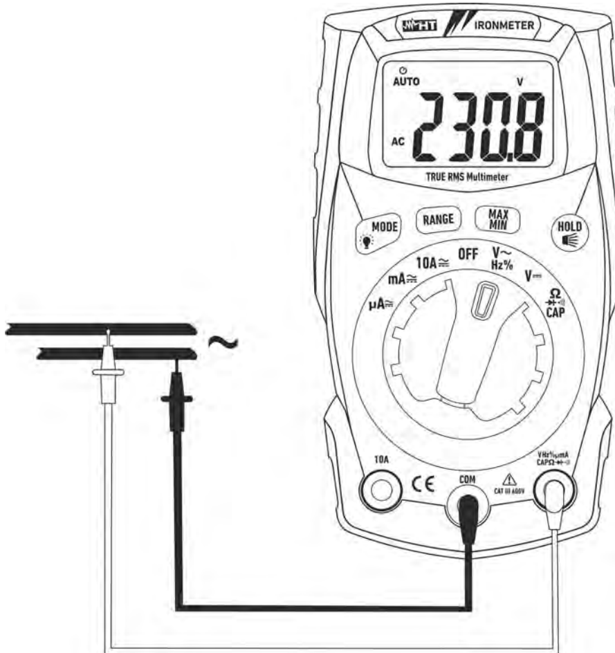
Fig. 4: Use of the instrument for AC voltage measurement
