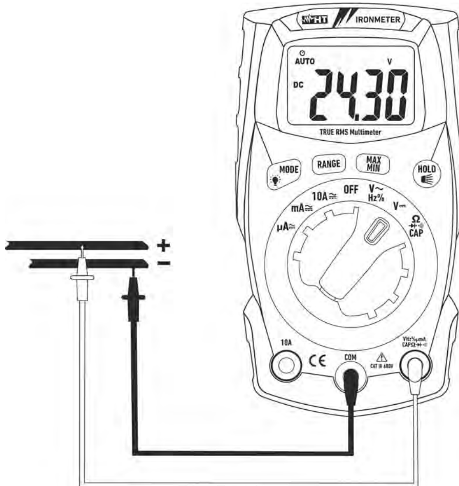
Fig. 3: Use of the instrument for DC voltage measurement
