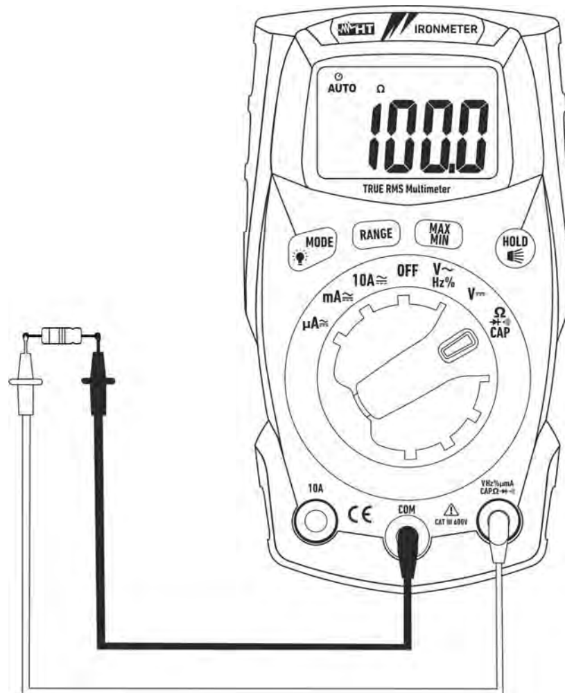
Fig. 5: Use of the instrument for resistance measurement and continuity test
