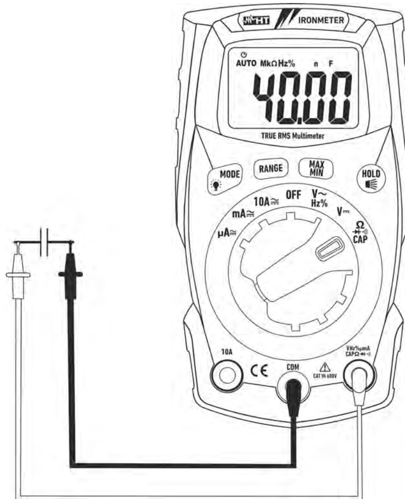
Fig. 7: Use of the instrument for capacitance measurement
